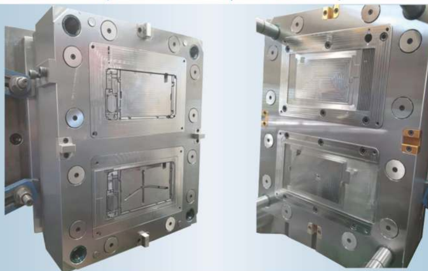
Stampo mostrina bi materia (ABS + PC/ABS) per strumentazione elettrica Mold for cover 2 plastic materials (ABS + PC/ABS) electrical field
